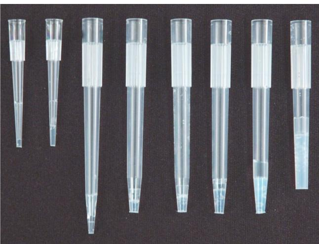
**PhyTip Columns.** Pictured from Left to Right. PhyTip columns packed with 5, 20, 10, 20, 40, 80, 160 and 320  $\mu\text{L}$  resin.
