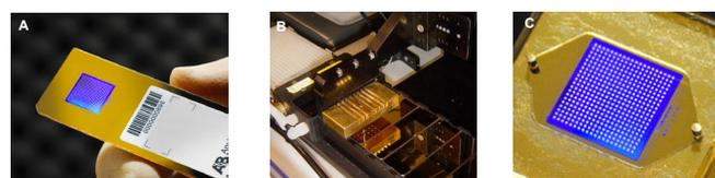
**Figure 2.** 8500 Affinity Chip containing 400 spots of protein depositing using conventional contact spotting robotic technology (A,B). Each spot is in the range of 150-250 microns in diameter, created by dispensing nanoliter volumes of protein onto the surface of the chip. The photograph shows the fully assembled chip and flow cell (C). The Affinity Chips are designed as single-use, disposable parts allowing affinity characterization of hundreds to thousands of interactions per day.
