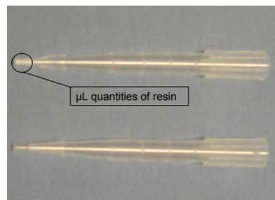
**Figure 3.** PhyTip™ columns are designed to encapsulate a small amount of resin within the end of a pipette tip. The dead volume if the column is kept to a minimum by suspending the resin between two screens, allowing for high enrichment at small volumes.
