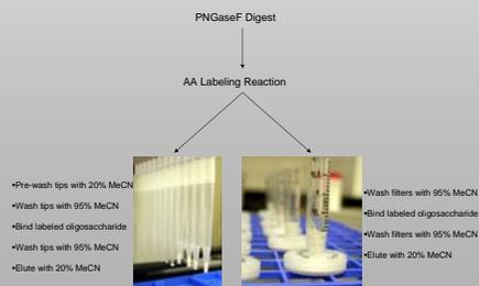
Figure 1. Schematic overview of the two oligosaccharide cleanup methods.
