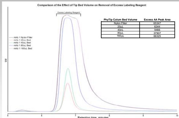
Figure 2. Labeled oligosaccharides were purified using Phynexus tips packed with 160 $\mu$ L, 80 $\mu$ L, 40 $\mu$ L or 20 $\mu$ L of DPA-6S resin and compared to a standard preparation from a nylon syringe filter. Injection volumes were 100 $\mu$ L for all samples.
