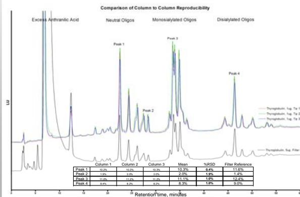
Figure 4. Thyroglobulin digests with purification on a 10 $\mu$ L Phynexus tip. All injections were 20 $\mu$ L. Sample preparations on three different tips gave super-imposable chromatograms. Peak area % observed were comparable to those obtained with nylon filter preparations with little variability from column to column.
