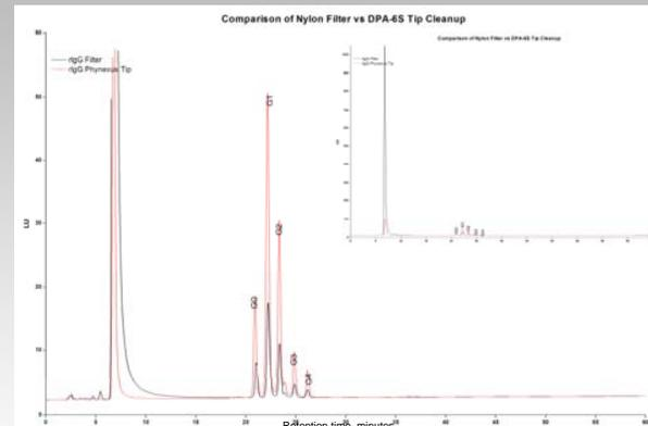
Figure 5. rIgG digests (5 $\mu$ g) with purification on either a 10 $\mu$ L Phynexus tip or a nylon syringe filter. Full scale chromatogram is shown as an inset. Both injections were 20 $\mu$ L (represents 20% for the PhyTip column and 2% for the nylon filter).
