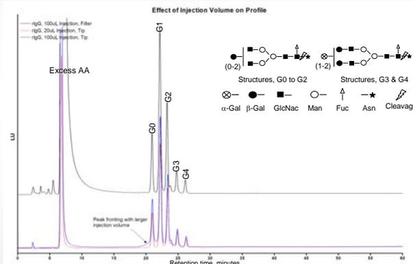
Figure 3. 5 $\mu$ g rIgG digest with purification on a 20 $\mu$ L Phynexus tip. Initial experiments were performed using a 100 $\mu$ L injection volume. This led to overloading of the column and peak fronting and loss of resolution of the neutral peaks. Reduction of the injection volume to 20 $\mu$ L eliminated this problem. This injection from the nylon syringe filter was 100 $\mu$ L.
