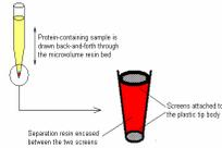
**Figure 1.** PhyTip™ columns are designed to encapsulate a small amount of resin within the end of a pipette tip. The dead volume if the column is kept to a minimum by suspending the resin between two screens, allowing for high enrichment at small volumes.
