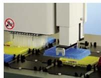
The ALH 3000 provides highly controlled reproducible flow rates for the 96 tip head. The Gripper removes and holds the lid from each plate.
