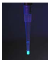
Fluorescently labeled IgG captured on the affinity resin of a PhyTip 200+ column
